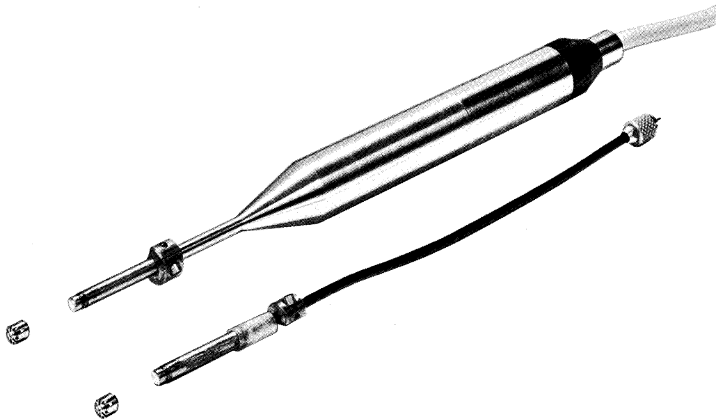
Fig.4. Receiver microphone with a specially low-stressed diaphragm and a low-noise preamplifier together with the transmitter microphone (a standard 1/8" Condenser Microphone Type 4138). The protecting grids are not used during measurements. The variable stops are used to position the microphones exactly in the reference plane
